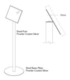
FullView Units are easily affixed to a 38mm diameter circular post at 1070mm via a modular steel mounting plate. The base plate acts as a counter weight at the bottom of the post. The FS300 can accept both Vertical and Horizontal display configurations - Check with APCO for size limitations.
