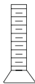
No. 6 x 25mm Flat HD Socket - SS Machine Screw for Base attachment
