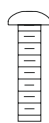
No. 6 x 25mm Pan HB Socket - SS Machine Screw for Sign Holder attachment
